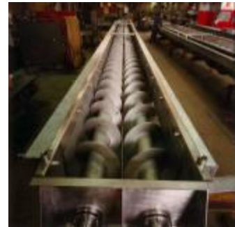
Screw conveyor bearings
