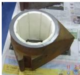
Peak cap bearing for Sedimentation Tank in Sewage treatment plant.
