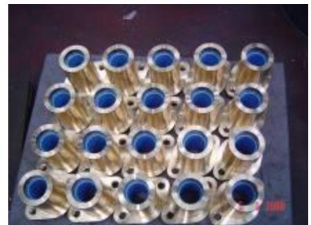
Lake Coleridge ThorPlas Wicket Gate bearings
