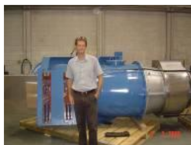
Thordon SXL Main Guide Bearings for Fereday Island Kaplan Generators.
